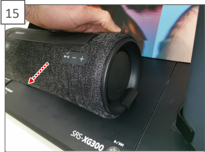
Slide the speaker forwards to lock it in place.
