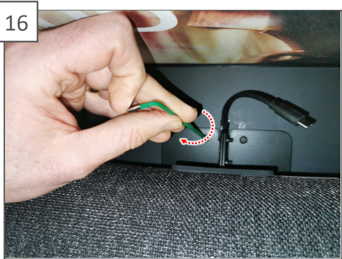
Re-fit the two screws at the rear of the speaker to prevent it from being slide back.
