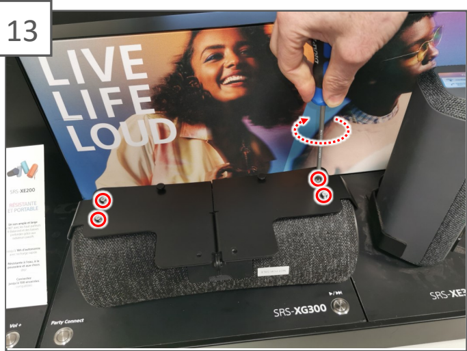
Re-fit the screws through the bracket into the feet of the new speaker.
