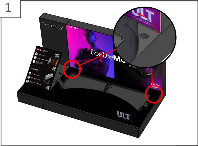
Peel back the back corners of the magnetic graphic to reveal the screws underneath.
